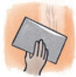
Surface imperfections such as holes, dents, fine cracks are to be filled with crack filler, before painting.
