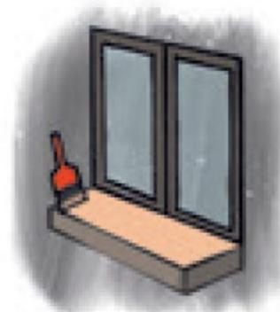
Ensure that horizontal surfaces like top of windows, ledges and other horizontal surfaces are painted with an additional coat for greater protection.
